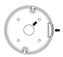
3 Attach the case-bottom to the mount bracket.
